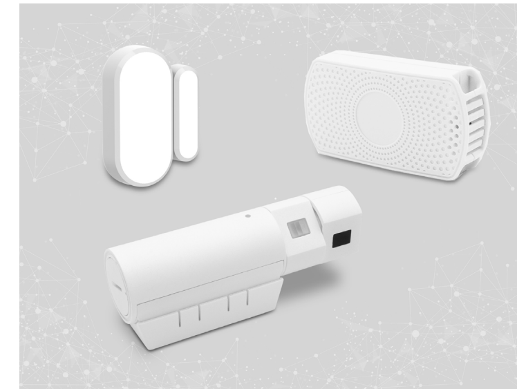
Sensor Beacons (Door Sensor, PIR/TOF Sensor, Temperature/Humidity)
